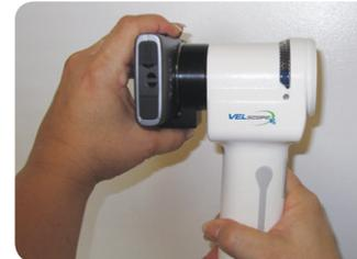
**3** Turn clockwise to fully lock the camera into the horizontal position.
