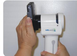
2 Engage the tabs on the camera bracket with the notches in the tube on the Handpiece.
