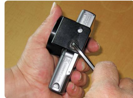
Screwing the bracket on properly ensures correct alignment with the camera. You can check the alignment by attaching the camera system to the Vx Handpiece and turning on the camera to deploy the lens. If the camera reports a "Lens Error...", then the bracket is not attached properly. If this happens, remove the bracket completely and reattach following the above instructions.
